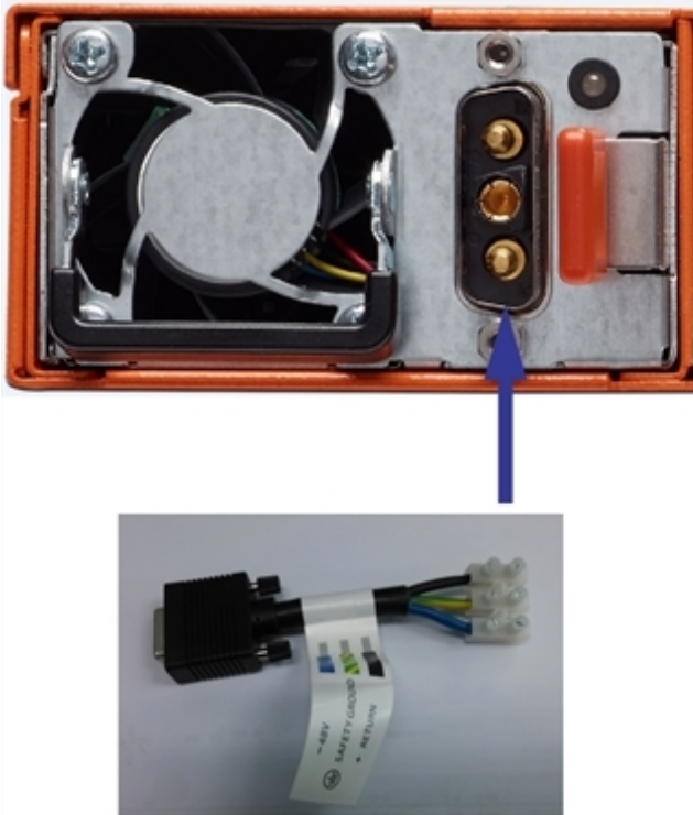
Figure 4 DC Power Module
